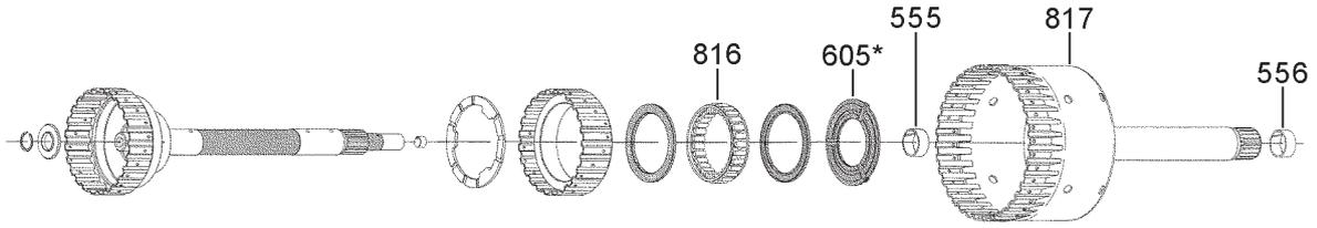
Forward Sprag, Direct Drum & Shaft Assy
